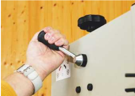
▲ A tensioning lever allows fast blade swaps
